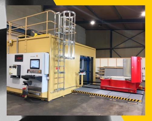
**XC05-2000-1R-450** is designed for automated handling of huge parts of aircraft engines. The system reaches its high level of functionality while being compact without any additional onsite concrete protection walls.
